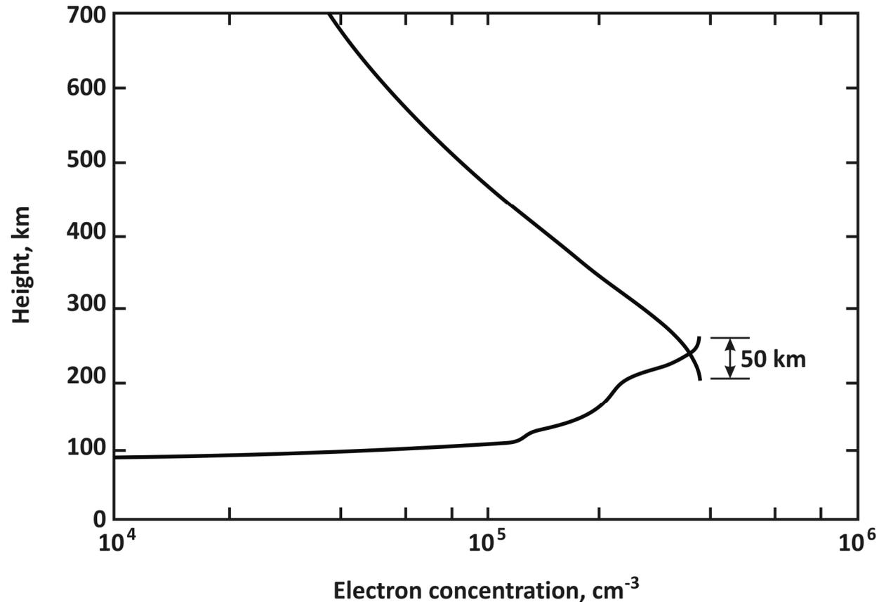
Fig. 5.5. [11] The distribution of electron concentration, obtained from the radio sounding of the ionospheric layers. This picture was obtained from the data of the external (from the satellite) and ground (from the bottom) radio sounding of the ionospheric layers.
