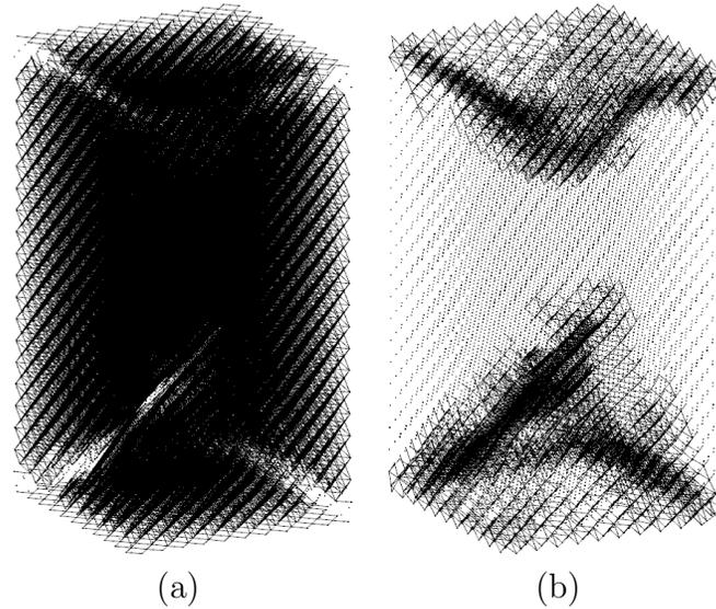
Fig. 2. Fracture pattern of solid ceramic specimen under compression: a) lines connect linked automata, b) lines connect unlinked automata
