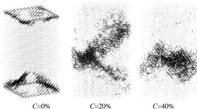
Fig. 3. First cracks in specimens with various values of porosity  $C$  under compression
