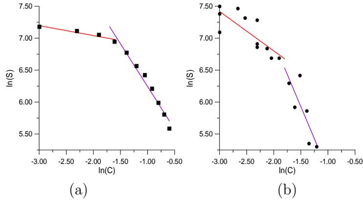
Fig. 7. Dependences of ceramics strength on porosity in logarithmic coordinates: a) simulation, b) experimental data
