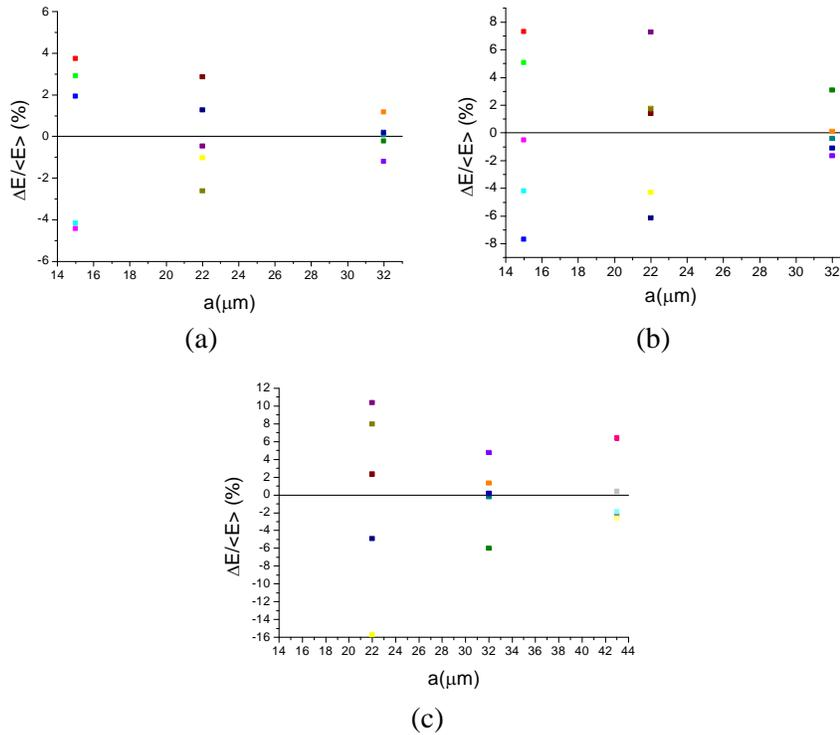
Fig. 4. Convergency of effective elastic moduli of the modeled specimens on their basis size for various porosity: a) 10 %, b) 25 %, c) 50 %
