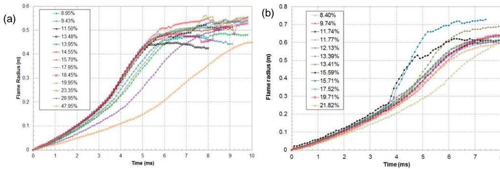
Figure 6. Summary of flame radius for different silane concentrations for (a) 0.3 m frame (b) 0.4 m frame.
