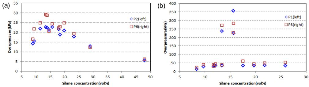
Figure 5. Summary of peak overpressures for different silane concentrations at different locations for (a) 0.3 m frame (b) 0.4 m frame.
