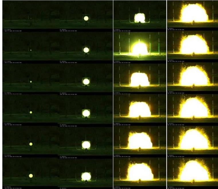
Figure 3. Typical results for flame propagation for different silane concentration 15.59 % in a 0.4 m cubic frame. Each frame differs by 0.3 ms.
