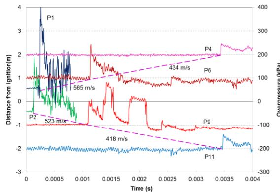
Figure 4. Overpressure histories of vapor explosion from silane concentration of 15.59 % in a 0.4 m cubic frame.
